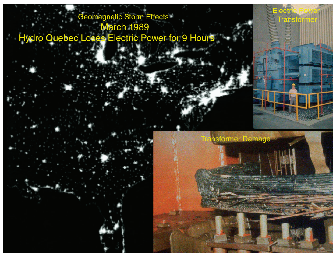
FIGURE 5.4 A 1989 geomagnetic storm caused a blackout in the Quebec region and damaged a high-voltage transformer. SOURCE: Rodney Viereck, NOAA Space Environment Center, “Space Weather: What Is It? How Will It Affect You?,” available at lasp.colorado.edu/~reu/summer-2007/presentations/SW_Intro_Viereck.ppt .
